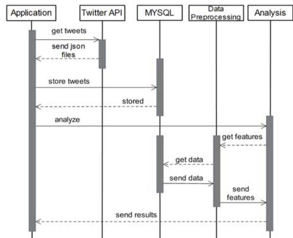
Fig. 2. The workflow sequence diagram.
