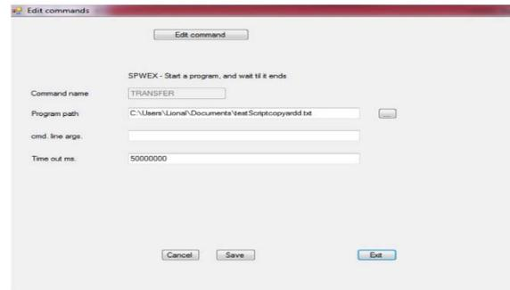
Fig. 4. Example of Gobetwino command allows transferring data from Arduino to host server
