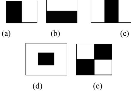
Fig. 2. Subset of Haar-like features prototypes. (a) Edge feature. (b) Line feature. (c) Center-surround feature. (d) Diagonal feature.
