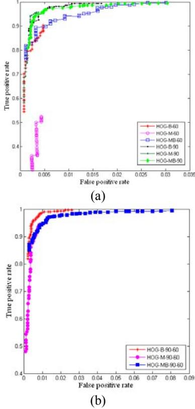
Fig. 5. The ROC curves of testing samples for traditional HOG method. (a) Non-mixed degree. (b) Mixed degree.
