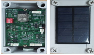
IoT sensor board prototype image
