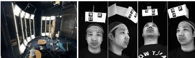
Fig. 1. (left) Our custom 4D facial-scanning rig; (right) synchronized multi-view images captured simultaneously.
