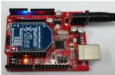
Fig.2. Arduino with Bluetooth module (FriBee)
