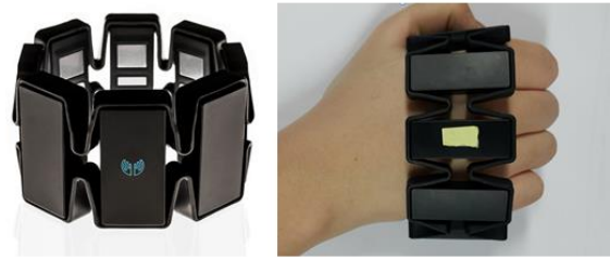
Fig. 4. Myo Armband (Thalmic Labs Inc) was held in a way that its sensor would be placed on the same location as those of retroreflective markers in Optitrack experiment.
